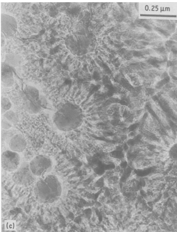
Figure 1 Powder microstructure. (a) Typical cross-section of medium-sized powder. (b) Dual microstructure morphology, microcellular–coarse cellular. (c) Coarse primary intermetallic particles acting as nucleation sites.
